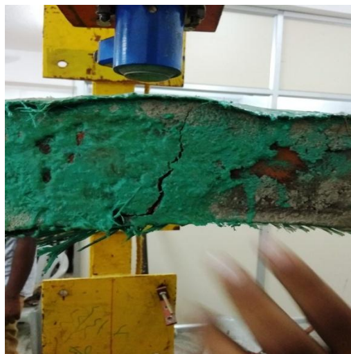
Fig 11: crack pattern on GFRP arches
