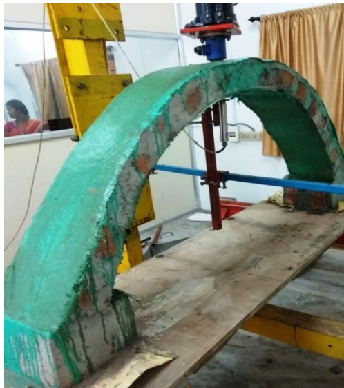
Fig 10: Testing of GFRP arches
