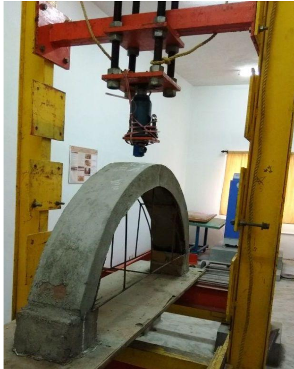
Fig 7: Loading Frame & Hydraulic jack attached to arch
