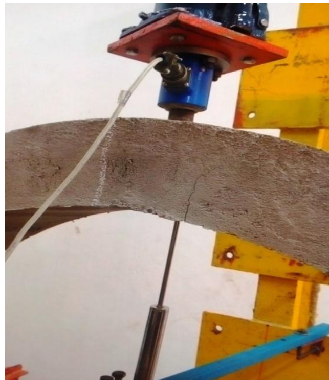
Fig 8: Initial cracks on arch
