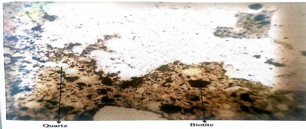
**Fig. 8** Plane view of shale sample (Ogb1-T) under photomicrography showing quartz, biotite and abundant of clay mineral
