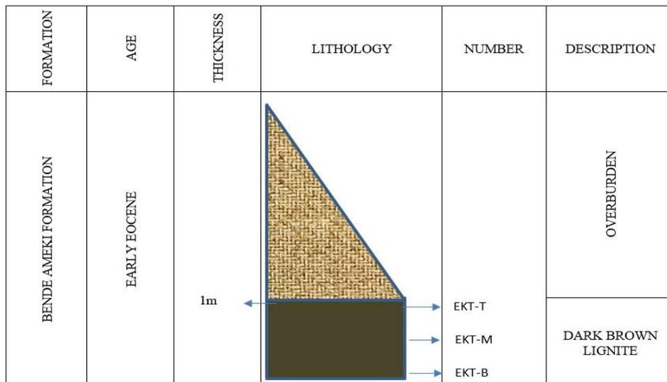
**Fig.3** Lithostratigraphic section of Bende Ameki Formation exposed at Eket spring in Umudiji
