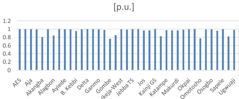
Figure 9.0: Nigeria 330kV Transmission Line Bus Voltage Profile During Occurrence of a Three Phase Fault on Ajaokuta Bus with ANN Controlled VSC-HVDC Installed
