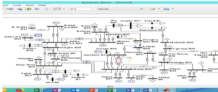
Figure 3.0: PSAT Model of the network when the VSC-HVDC is installed along Ajaokuta – Benin Transmission Line
