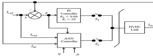
Figure 2.0: A schematic diagram of an HVDC system generic controller
