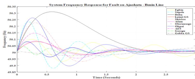
Fig 8.0: Frequency response of the system generators for fault clearing time of 0.5sec (with ANN Controlled VSC-HVDC)
