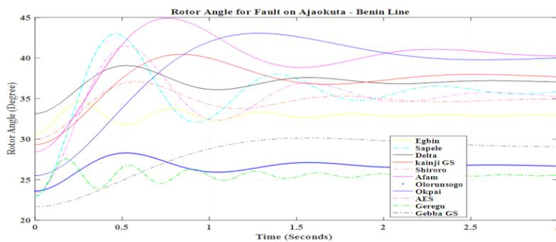
Fig 7.0: Rotor Angle response of the generators for fault clearing time of 0.5sec (with ANN Controlled VSC-HVDC)
