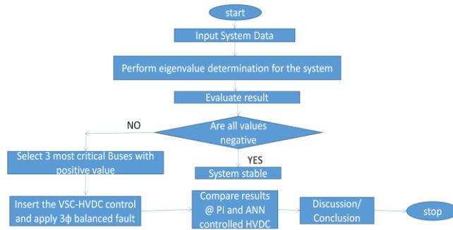
Figure 1.0: Flowchart for determination of Transient stability using Eigenvalue method
