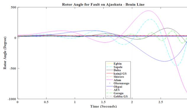
Fig 4.0: Rotor Angle response of the generators for fault clearing time of 0.35sec (without any VSC-HVDC)
