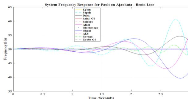
Fig 5.0: Frequency response of the system generators for fault clearing time of 0.35sec (without any VSC-HVDC)
