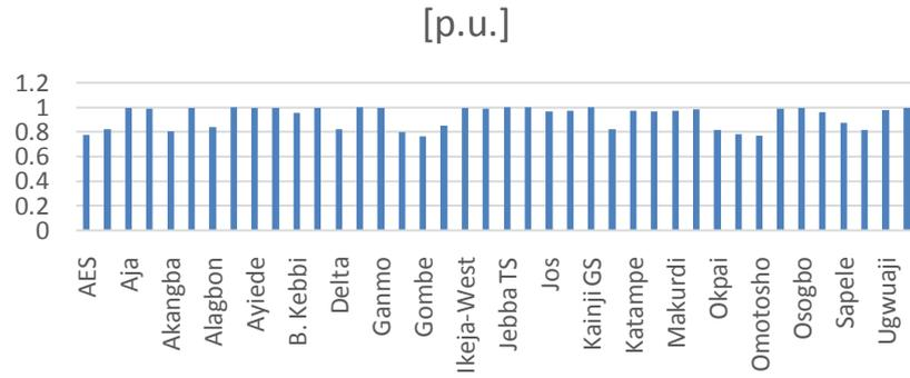
Figure 6.0: Nigeria 330kV Transmission Line Bus Voltage Profile During Occurrence of a Three Phase Fault on Ajaokuta Bus
