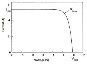
The I-V characteristics of a typical solar cell are as shown in the Figure 3.2.
