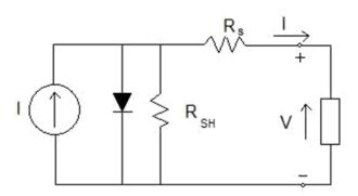
In this model we consider a current source (I) along with a diode and series resistance (Rs). The shunt resistance (RSH) in parallel is very high, has a negligible effect and can be neglected.
