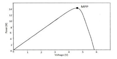
**3.4 Boost Converter** As stated in the introduction, the maximum power point tracking is basically a load matching problem. In order to change the input resistance of the panel to match the load resistance (by varying the duty cycle), a DC to DC converter is required.
