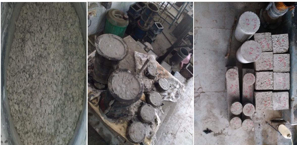
Fig. 4 Mixing, Casting, Curing of Geopolymer concrete
