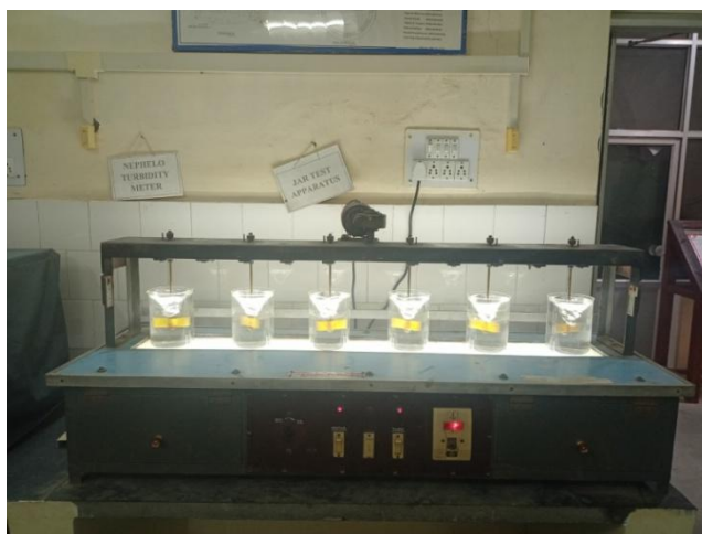
Figure-2: Jar test apparatus in collage laboratory, JEC Jabalpur M.P.
