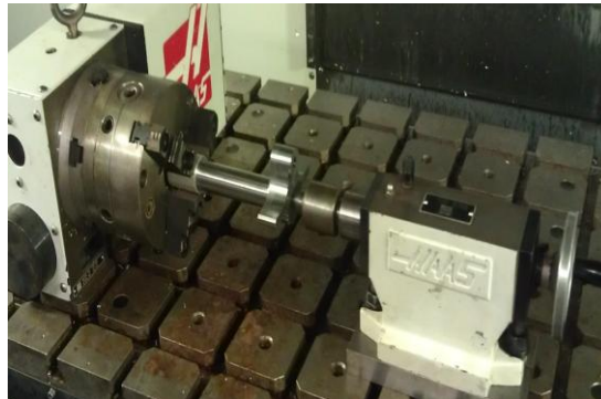
Fig.3.1: Crank-Shaft Fixtured for 4th Axis Machining
