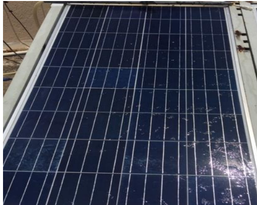
Figure 3.1 Front Surface Cooling by water
