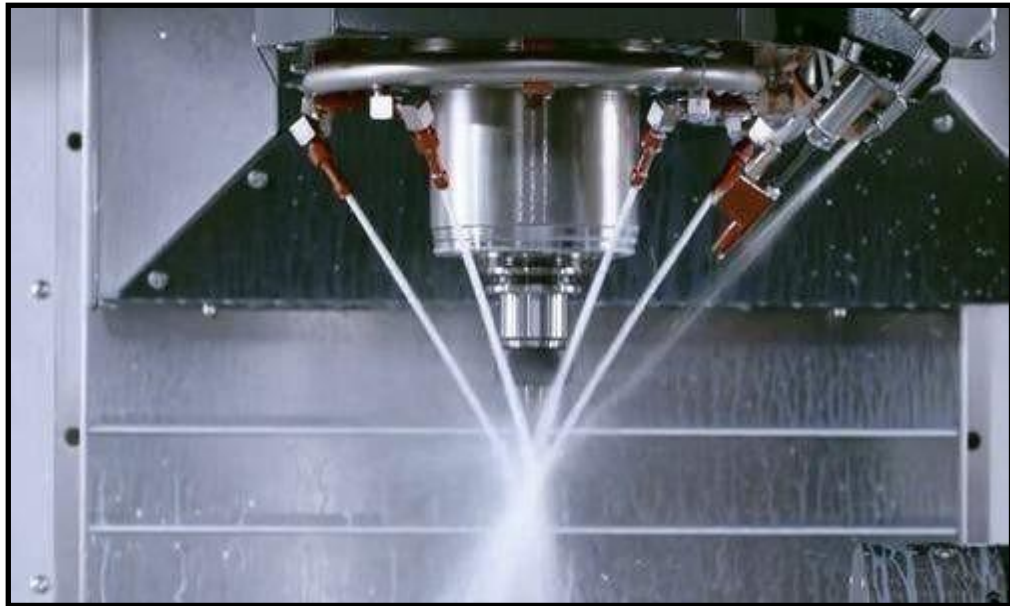
Fig.3.3.3 High Pressure cooling
