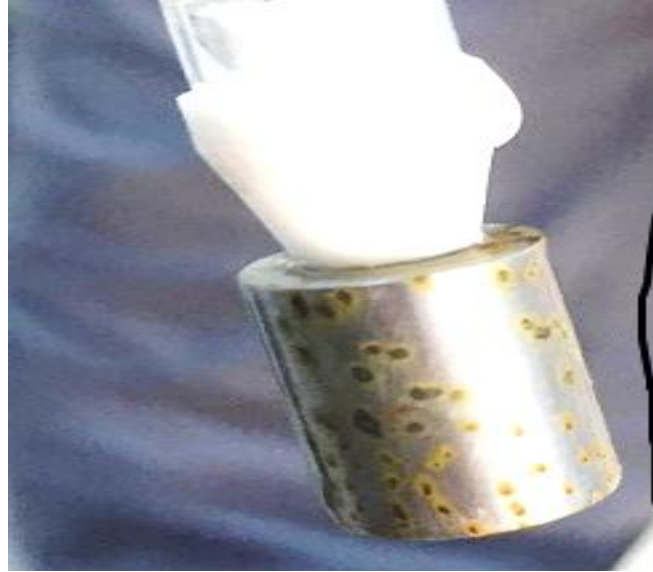
Figure 14 Examination of the Electrode Surface After Experiments at pH6 [Visible Pits ]
