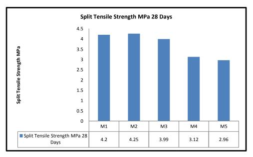
From the above test results and the graphical variation as shown in Table 4.4 and Fig 4.2, it was observed that the split tensile strength results of the M2 and M3 are comparable with the mix M1.
