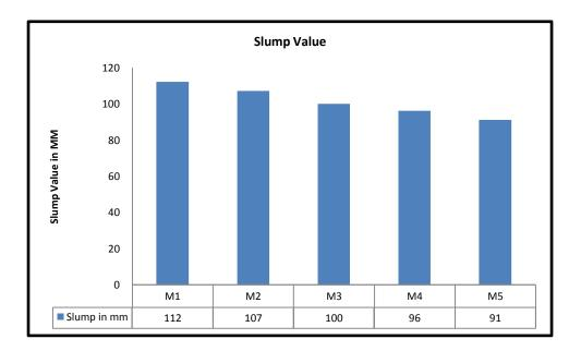
Table 4.2 shows that as the percentage of recycled concrete in the mix increases, the slump value decreases. This is due to the presence of dust and mortar on the surface of recycled aggregates, which causes them to absorb more water than conventional aggregates. By changing the super plasticizer dosage, all slump values were kept between 90 and 110 mm.
