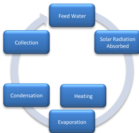
Fig 2: Flow chart on process of solar distillation
