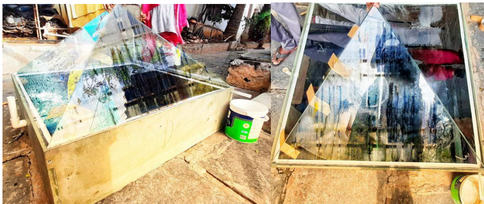
Fig 9: Pyramidal solar still at condensing stage.
