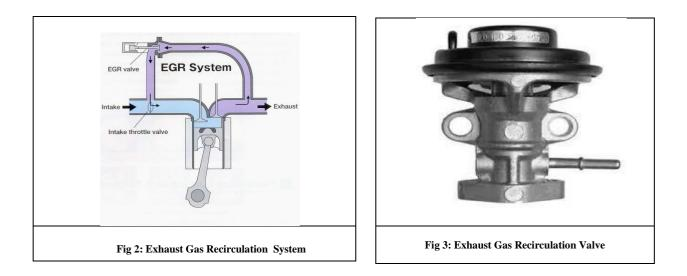
The purpose of the exhaust gas recirculation valve (EGR) is to meter a small amount of exhaust gas into the intake system; this dilutes the air/fuel mixture so as to lower the combustion chamber temperature. Excessive combustion chamber temperature creates oxides of nitrogen, which is a major pollutant. While the EGR valve is the most effective method of controlling oxides of nitrogen, in it's very design it adversely affects engine performance.
