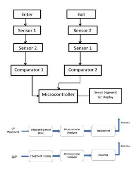
For counting and measuring the distance we made two methods: measureDistance() and calculateDistance(). We set The Particular Distance (Depend on the Door Size). The Sensor Attached at a point that can Detect the person who is Passes from door or not. The all Sensor Are Connected to the main Machine which is present at HOD Room Where is Monitoring the labs. These sensors signals are transmits in encrypted way. For Transmission We are using NRF module.
